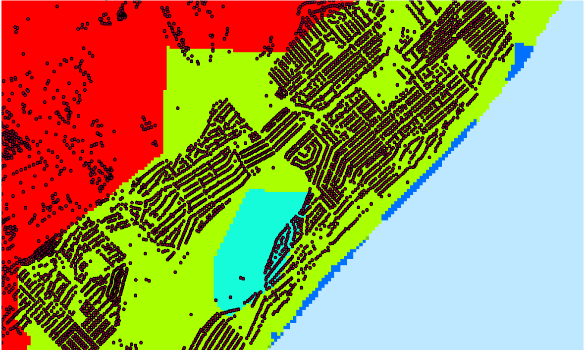
Figure 3: Coastal Development areas are still marked as natural areas on NLC 2000 Urban Areas (Red), Natural Areas (Green), Waterbodies (blue), ESKOM SBC (dots).
